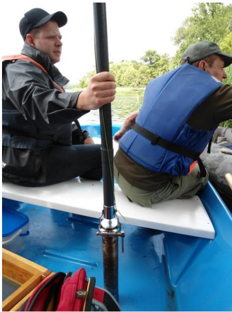
Figure 3.: „Kajak”- sampler for sediment collection in deeper parts of the lake
