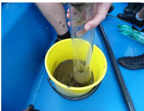
Figure 6.: taking the sediment samples on board
