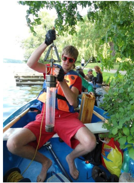
Figure 4.: „czapla” sampler for the collection of sediments from the shallower parts of the lake
